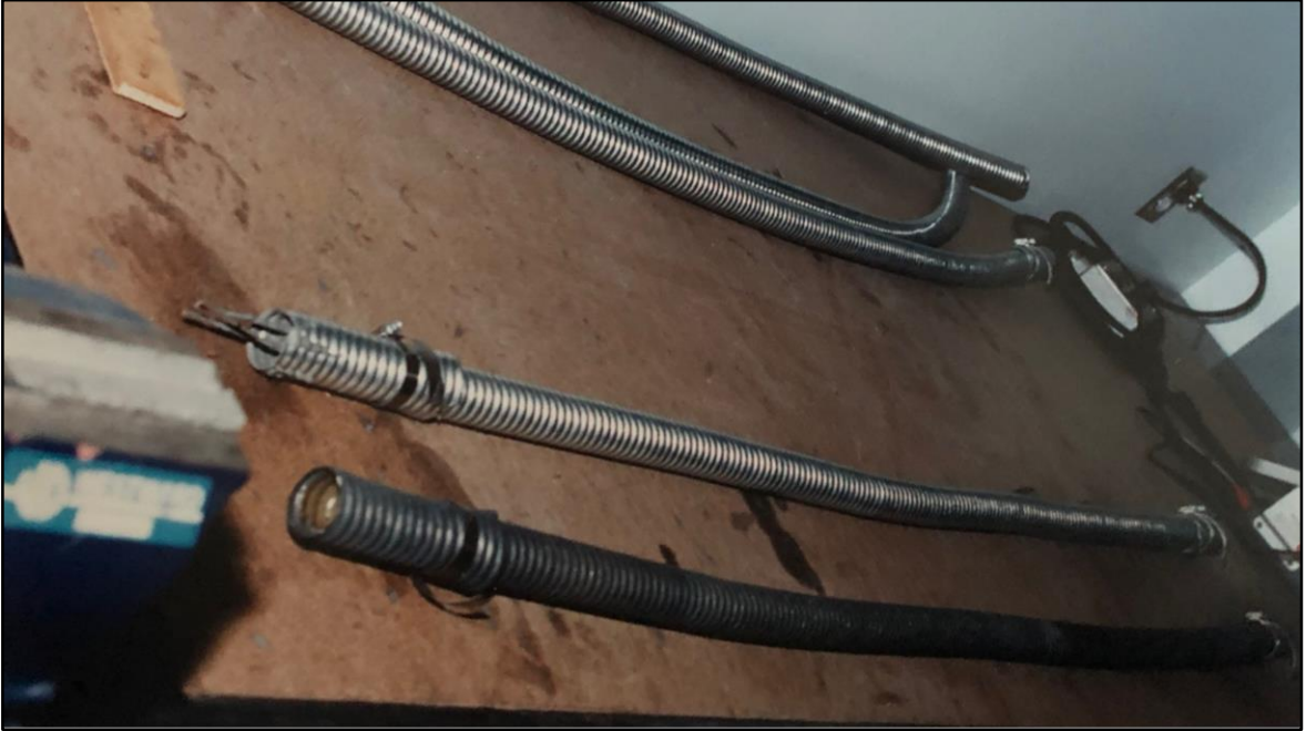
This is armored pump cable. It is used to power submersible pumps in oil wells far underground.
