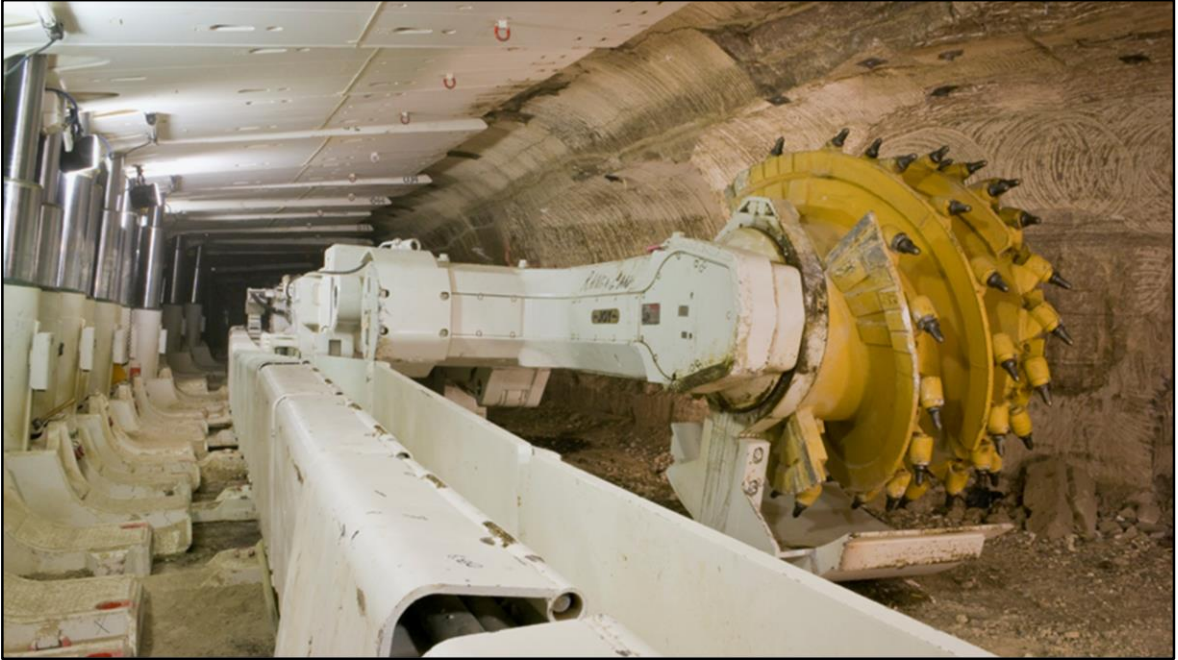
This is a long wall machine at a trona mine in Wyoming. 1700 feet underground. There is nothing but those hydraulic jacks on the left to hold the roof up.
